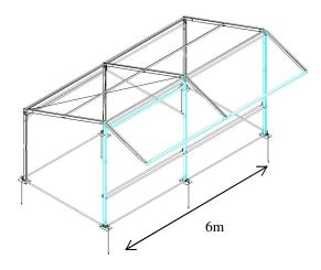
The Sales Stall is designed to provide a weatherproof structure optimised for use as a sales counter for outdoor events. The aluminium frame and PVC covers allow quick and easy assembly by two people.
