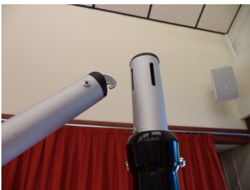
Hook horizontal pole into slits on vertical pole
