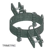
5. Attach lower pulleys to opposite sides of bail ring, passing lifting tail of rope between bail ring and king pole. Thus when lifting the bail ring, the end of the lifting rope is between the ring and the king pole.
