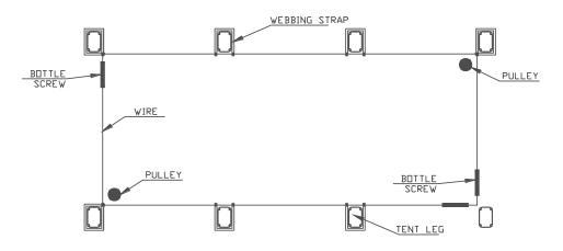
Make sure bottlescrew is fully opened and hook on to wires at opposite corners. Pull wire tight through bottlescrew then tighten clamps. Close bottlescrew as tight as possible to tension the wire.
