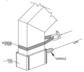
Pull up the lifting poles to shoulder height, and then attach the roof extensions by tying the webbing straps in a bow like a shoelace. Repeat on every bay. Attach each roof to it's neighbour and pull down the length of the ridge to get a taut straight line. Attach the gable to the roofs at each end ensuring that the webbing is secured to the lifting bar. To attach a hip end there is a webbing strap with an eyelet through. Tie this around the end of the lifting pole.
